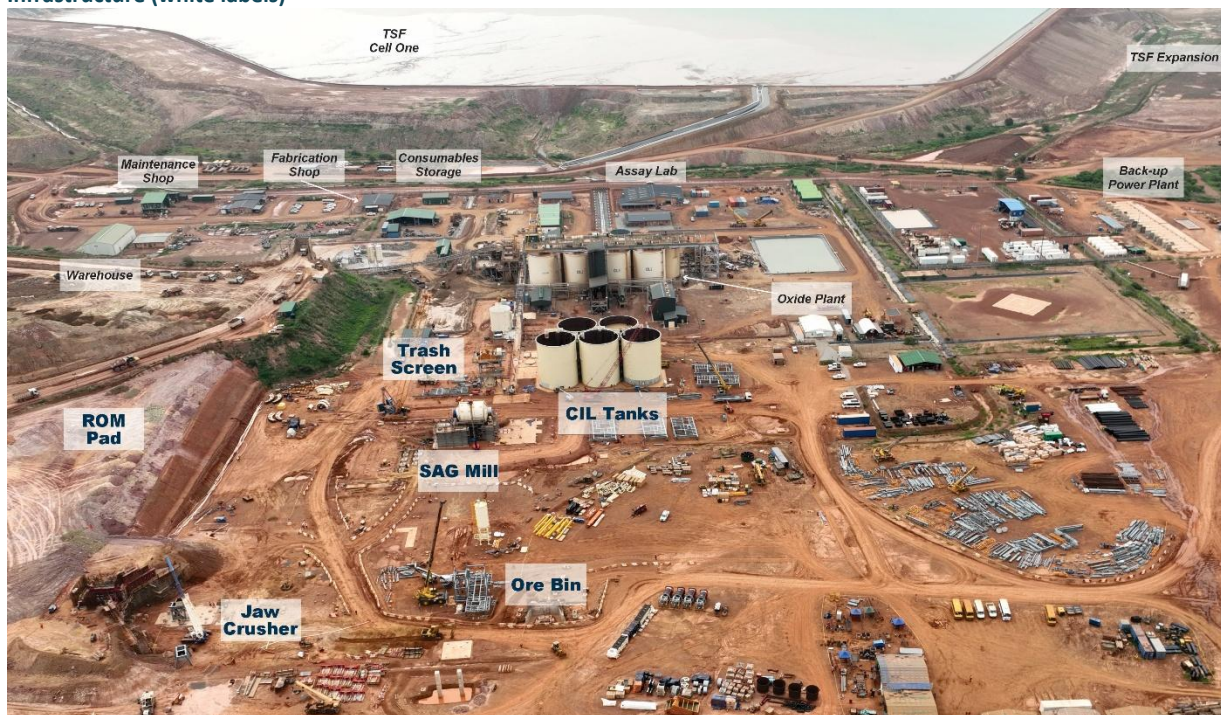
Figure 1: Bomboré Processing Complex – Hard Rock Plant Layout (blue labels) Relative to Oxide Plant and Other Established Infrastructure (white labels)
