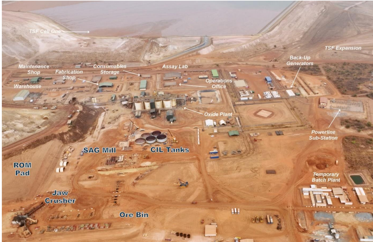
Figure 1: Bomboré Processing Complex – Hard Rock Plant Layout (blue labels) Relative to Oxide Plant and Other Established Infrastructure (white labels)
